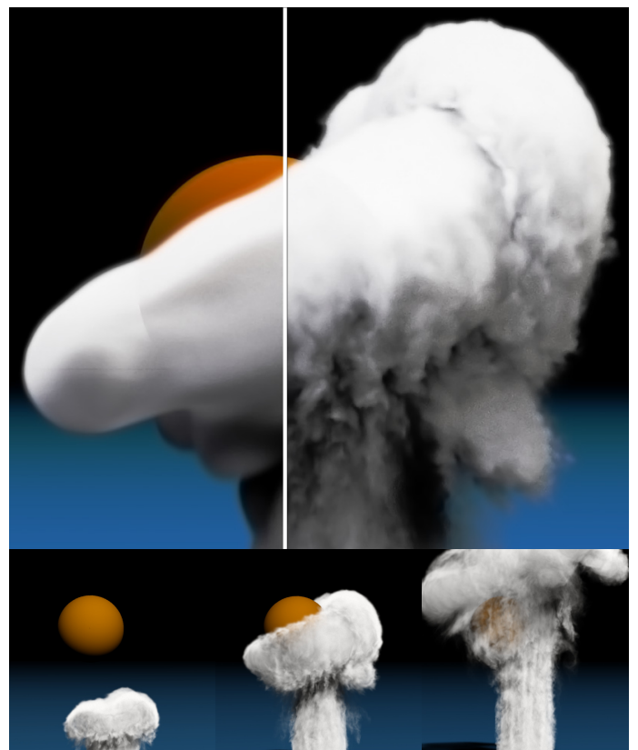
Figure 6: Flow around a sphere with grid-based densities. The low resolution simulation is shown in the left half of the top image. Wavelet turbulence synthesized a 400^3 grid from a 50^3 grid. Each frame took an of average 30 seconds on a four core workstation.
